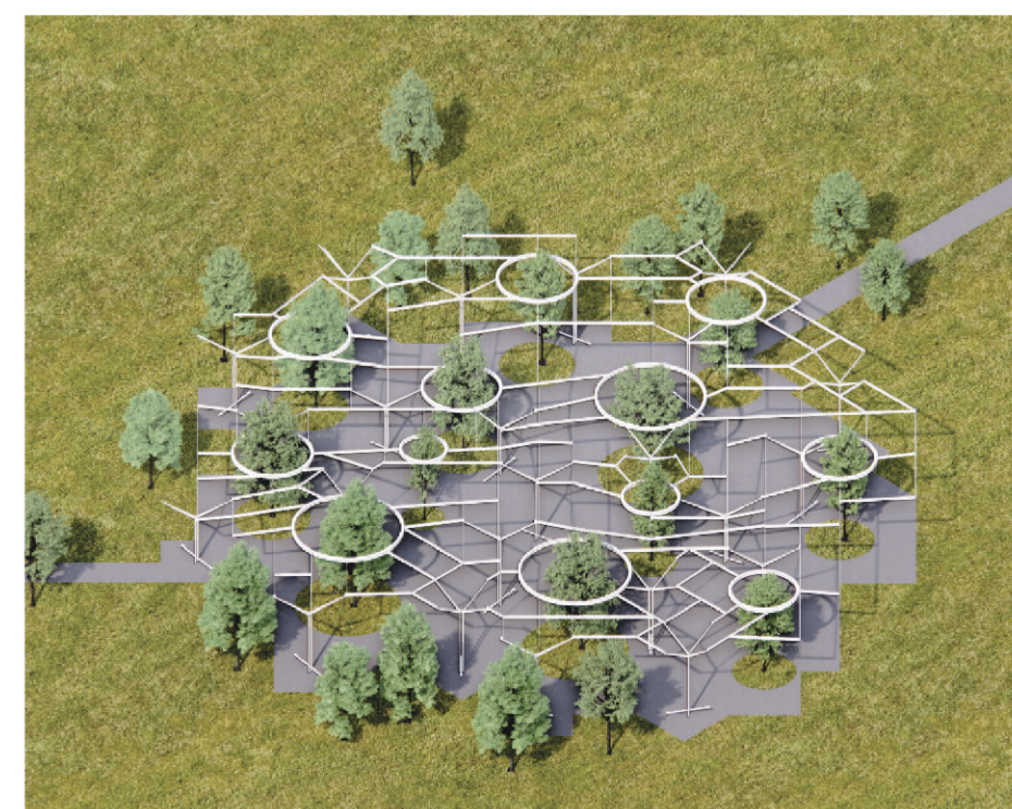
3. Linear and circular beams connect vertical structures
