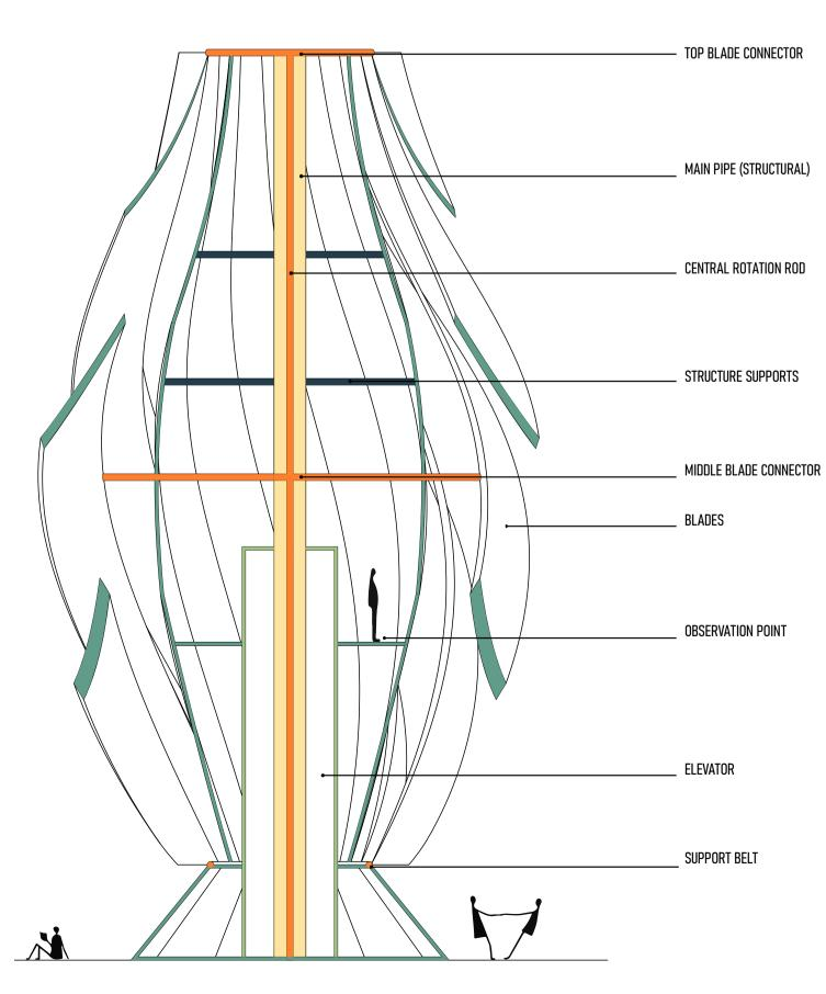
Wind Turbines-Observation Section | Scale 1:125
