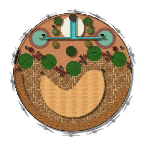
This design is designed as an independent pavilion. The project generates electricity using solar panels on the roof, smart flooring, wind turbines and a water mill.
