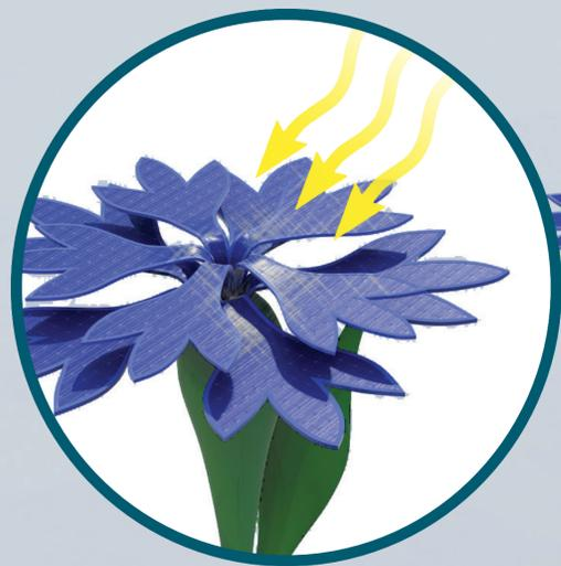
Energy from sun rays is absorbed by the photovoltaic cells in the petals and converted into electrical charges resulting in energy flow
