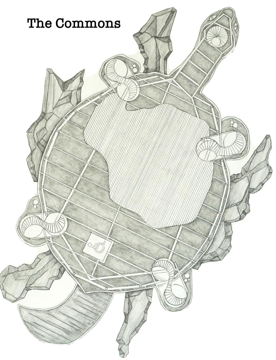
The Commons are 28 m long and 23 m wide constituting 371 sq m of reclaimed floor joist decking. Includes ADA accessible lift.
