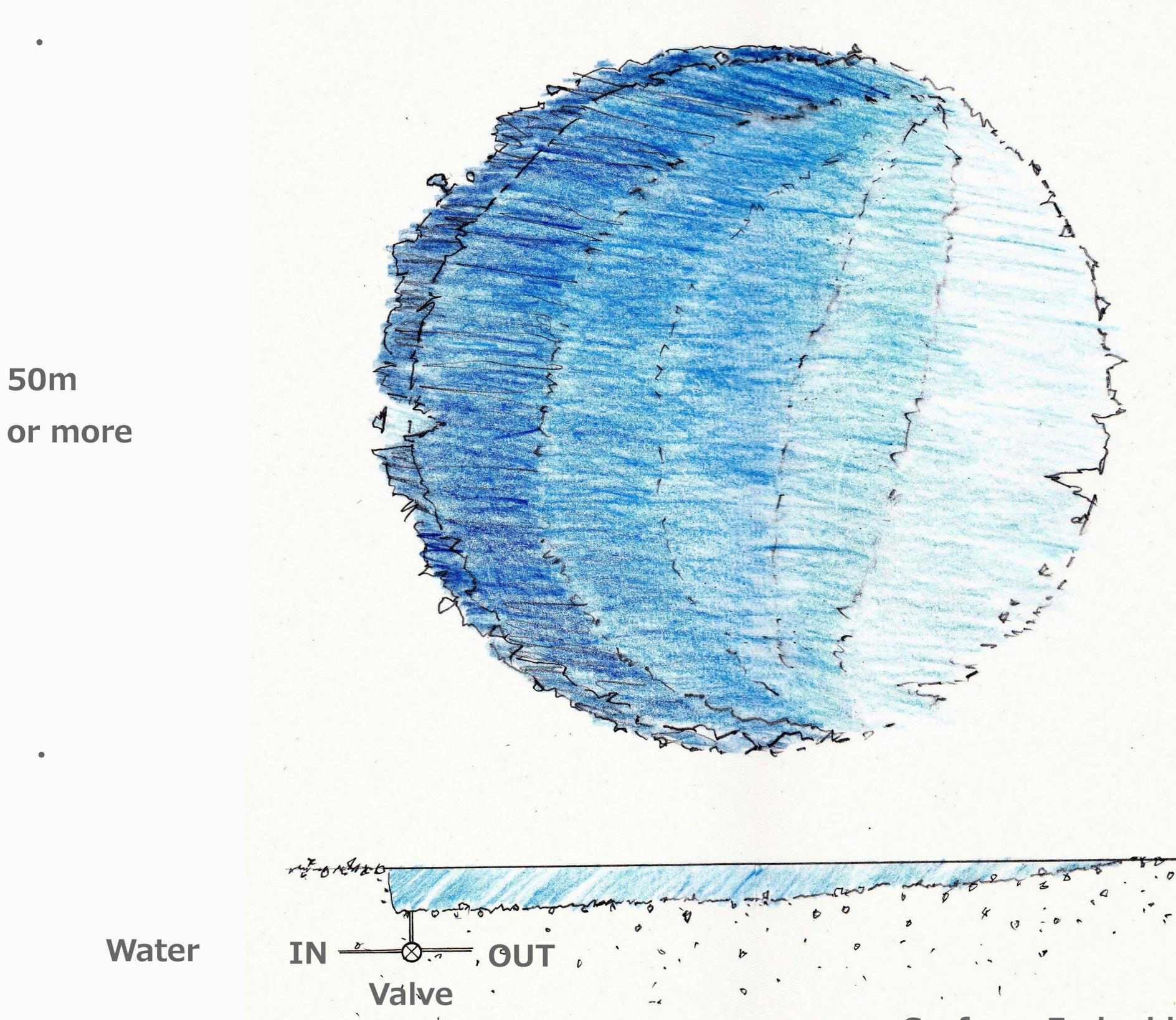
Surface- Embedding stones, sand and soil. Base- Waterproof mortar.
