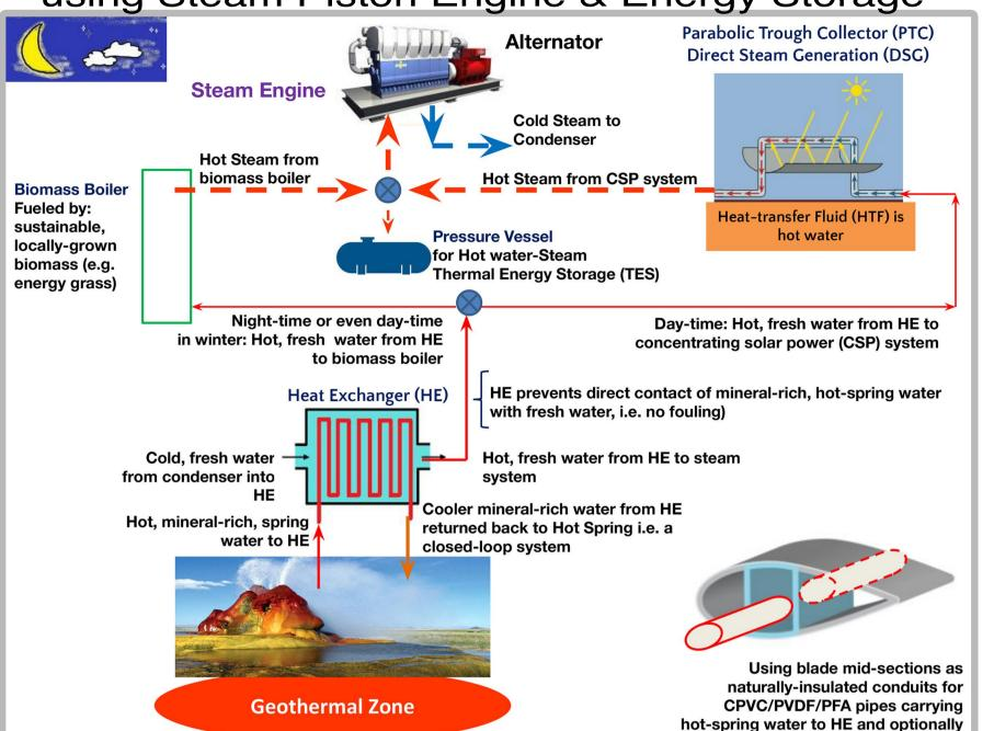
3. Solar-Biomass-Thermal Hybrid Power Plant using Steam Piston Engine & Thermal Energy Storage
