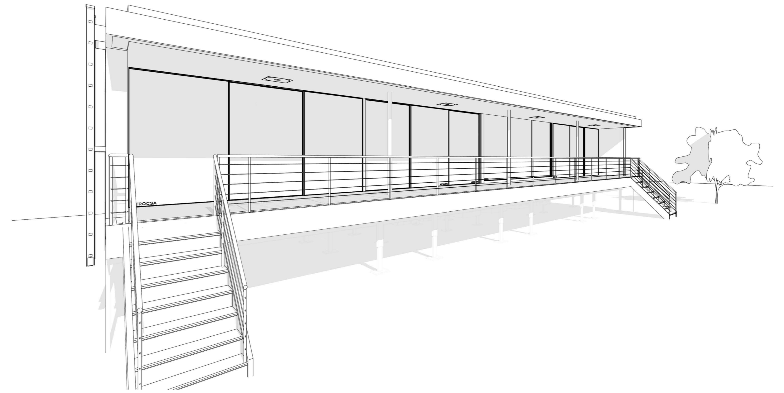
Patio is located on the southern face of the building to provide solar shade during the summer months
