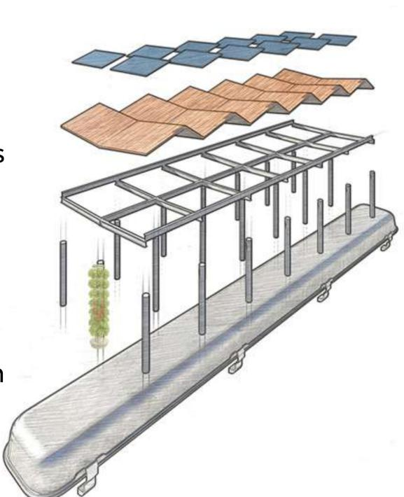
The structure centers on a multifunctional roof that generates solar power, collects rainwater, and provides shelter. Supported by a modular steel frame, the
