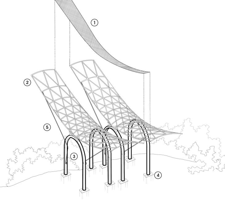
1 Fog catcher between structure (woven high-density polyethylene -HDPE- mesh) 2 Bamboo structure 3 Brass arches 4 Foundations 5
