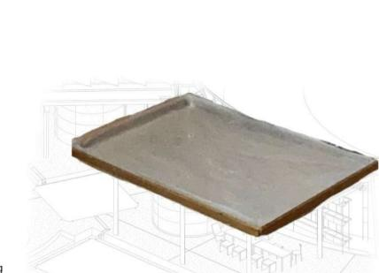
A plastic film as 1st waterproof layer cover all faces except the ceiling, needing to cut corners and then seal it with silver tape. Pipe type B. is exemplified to show how the film bends into it. The timber slab thus receives an hermetic layer. The fascias sides will be protected with an aluminum flashing and, if rain occurs with wind, with a varnish, only in these parts.
