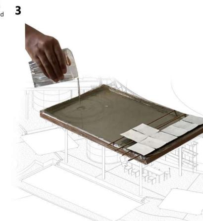
Few hours after, potable water fills the bowl till 40cm h to complete the semilightweight slab-water roof. Partially covered to foster curing for 14 days, water is lowered to designed 35cm, and 5cm h aluminum railings with pedestals are set to reinforce solar PV modules
