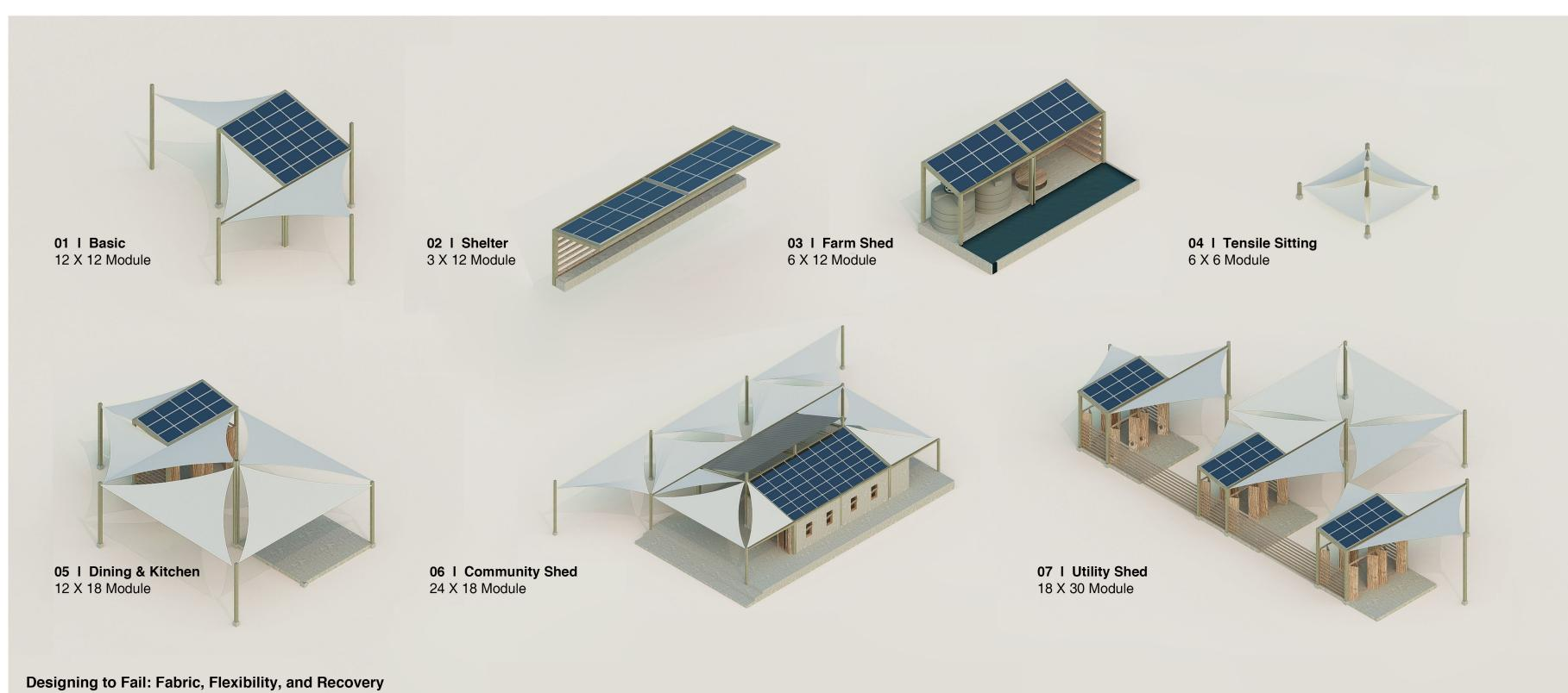
Central to the architectural language is a tensile canopy system designed with intentional impermanence. Lightweight membranes are engineered to disengage or collapse under extreme weather, minimizing structural damage and
