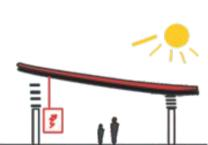
SHEET ROOF WITH STRUCTURE WITH FLEXIBLE SOLAR PANELS WHICH ADAPT TO THE SHAPE OF THE ROOF, EACH BUILDING IS SELF-SUSTAINABLE AND HAS THE POSSIBILITY OF STORING ELECTRICAL ENERGY IN INTERNAL BATTERIES.
