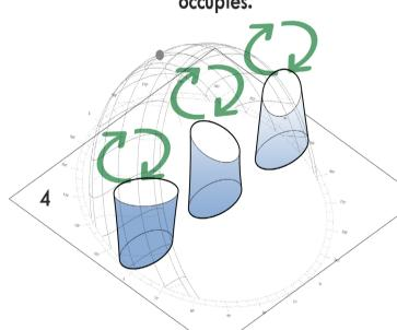
Using SMA materials as arms that change shape to modify the structure at the top and increase the solar collection area.
