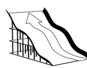
The lowest edge of the slope integrates with the ground and faces the direction of incoming hurricanes, enhancing the structure's stability and resilience.
