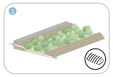
**Patch: Treatment Planter** Runoff infiltrates and is naturally cleansed through soil and vegetation
