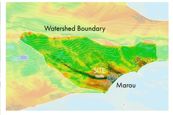
The site has a large watershed and clean rainwater due to dense forest coverage and a clean atmosphere. However, the upper areas of the site have steep slopes of up to 50%, posing risks of soil erosion and sediment runoff. Additionally, the site acts as a floodplain during storm events. So it provides both opportunities and challenges for water management.
