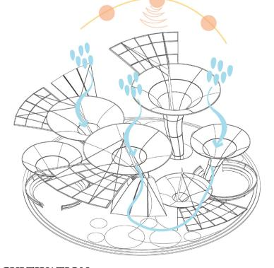
One of the most important elements of our project is the funnels that collect rainwater and water from precipitation. They are made of fibreglass and are designed to collect water for the residents. Underneath them are water collection tanks. The water is constantly circulating
