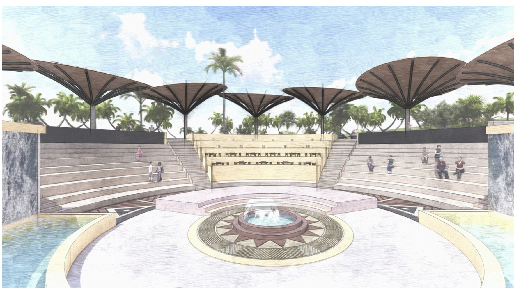
Image of what it's like literally inside the "Kava bowl" on the far end from the front, we have the shaded pavilion area that is inspired by the Kava leaf design. These structures act as solar shading, they host the solar panels above, as well as act as rain water catchment, harvesting water and leading it to underground water tank.
