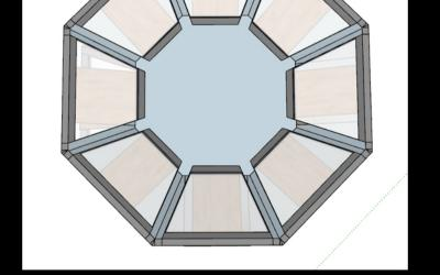
Design . Octagonal building single plane shape, easy to modular development, easy to local residents construction, but also suitable for factory prefabrication production
