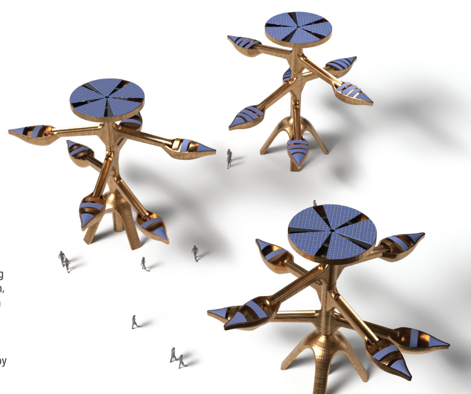
The Fiji project blends sustainable energy and water collection with organic-nature inspired design. Using locally sourced material where applicable, Aluminum, stainless steel, and photovoltaic panels. This system integrates a solar canopy with water collecting leaf-like structures along the tree's sculpture. At its base lies a gathering area shaded by the leaf shaped panels above and provides seating for people to enjoy the beautiful Fiji rays.
