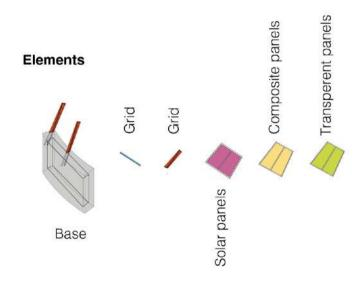
The station structure is assembled at the construction site from ready-made elements as a construction kit. Each of the modules has a low weight, the material of the spatial frame is aluminum.
