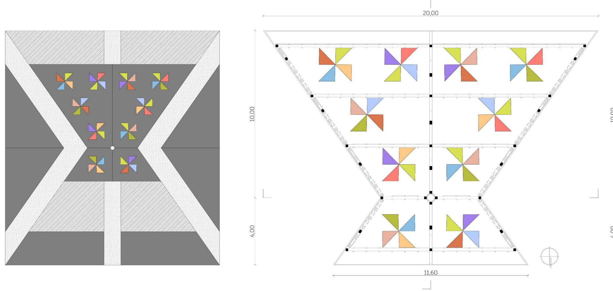
The central building has two levels: the lower level houses the mechanical room, the water collection tank, a multifunctional water block and agricultural storage. The upper level is open and can be used flexibly as a community space, training area, processing area or temporary accommodation. The roof structure is a solar panel array on lightweight lattice supports, which both generates electricity for the main building and captures and collects rainwater for the tank.
