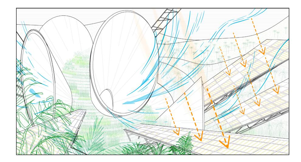
Solar & Wind Synergy: The installation's sweeping sail arrays (250 m² per unit) serve a dual highefficiency purpose: Solar Harvesting - Photovoltaic-coated surfaces generate 15-25 kWh/day (depending on climate), powering:
