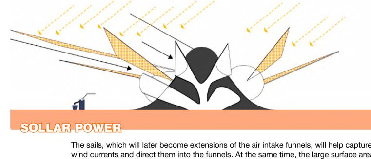
The sails, which will later become extensions of the air intake funnels, will help capture wind currents and direct them into the funnels. At the same time, the large surface area of the sails allows us to install solar panels on them. For a single unit, the total sail area is approximately 250 m², and depending on conditions, one square meter of solar panels can generate varying amounts of energy per day.
