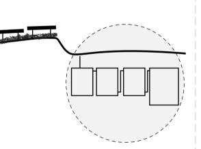
We propose a natural water filtration system that utilizes rocks, sand, and coconut fiber. Rainwater is collected through concave-shaped features and then filtered in an underground tank. The clean, filtered water is stored and distributed to the village using pump-powered energy.
