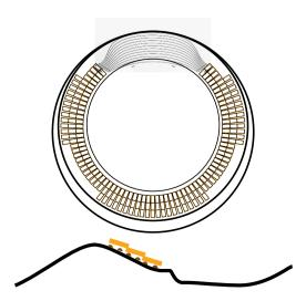
4 - COVER the slopped terrain with standard photovoltaic ,anchored on bamboo trunks
