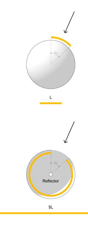
Diagram showing the difference in area according to installation location of solar cell based on average sunshine hours (4 hours)
