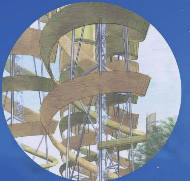
The skin of the spiral structure comprises approximately 18000 of integrated photovoltaic and flexible mono-crystalline silicon photovoltaic panels.
