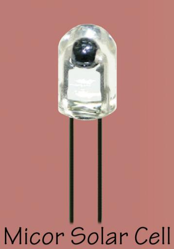
The spherical micro solar cell is encapsulated with plastic moulding. This micro solar cell has 360° view angle that captures the light from all directions. It has a maximum power point of 0.66 mW and an efficiency of 25.9%.
