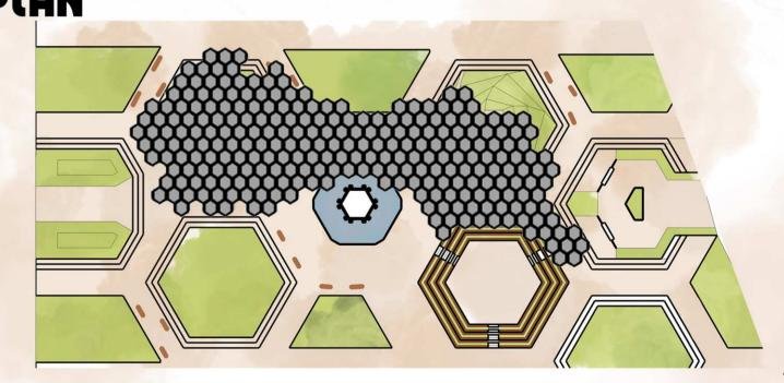
A CANOPY CONSISTS 937 PIECES OF HEXAGONAL BLOCKS (THE AREA IS 5.8M2 EACH) WITH SOLAR BATTERIES.
