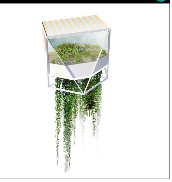
The Oasis module is made of a **white steel structure**, a hermetic glass panel topped by a translucent solar panel, some earth and substrat, a line of bioluminescence and plants. All modules can be either independant, or connected with an other .
