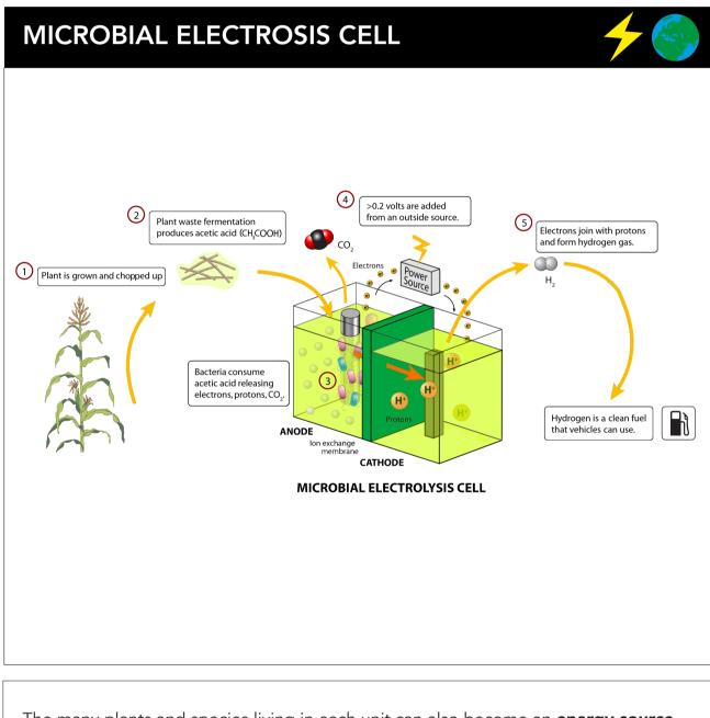
The many plants and species living in each unit can also become an **energy source**, thanks to the microbial electrolysis cells placed in the dirt. This System produce also Hydrogen for vehicules
