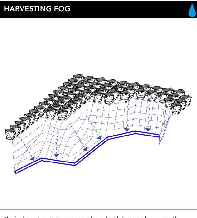
This fog harvesting device is composed by a **double layer mesh**, supported by the Oasis module . The collectors are **oriented in various directions**, always perpandicular to the ground, maximizing the capture of precious water .
