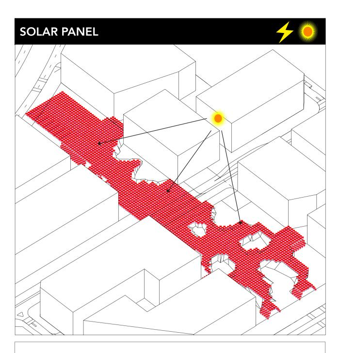
All the Solar Panel are made from the ASCA film : it's a **flexible** film that can be put on a glass panel and is **translucent** . This panel can measure up to 6 meters long and 60cm large, and is **extremly light** : 450g/m2 . The maximum energy is 80Wc/m2
