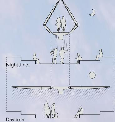
At nighttime the leaves retract and give away the view to the nightsky. Embedded OLEDs create a light tunnel which shines throught the flooring, reflecting the motion of people via the Tyndall effect under the bridge.
