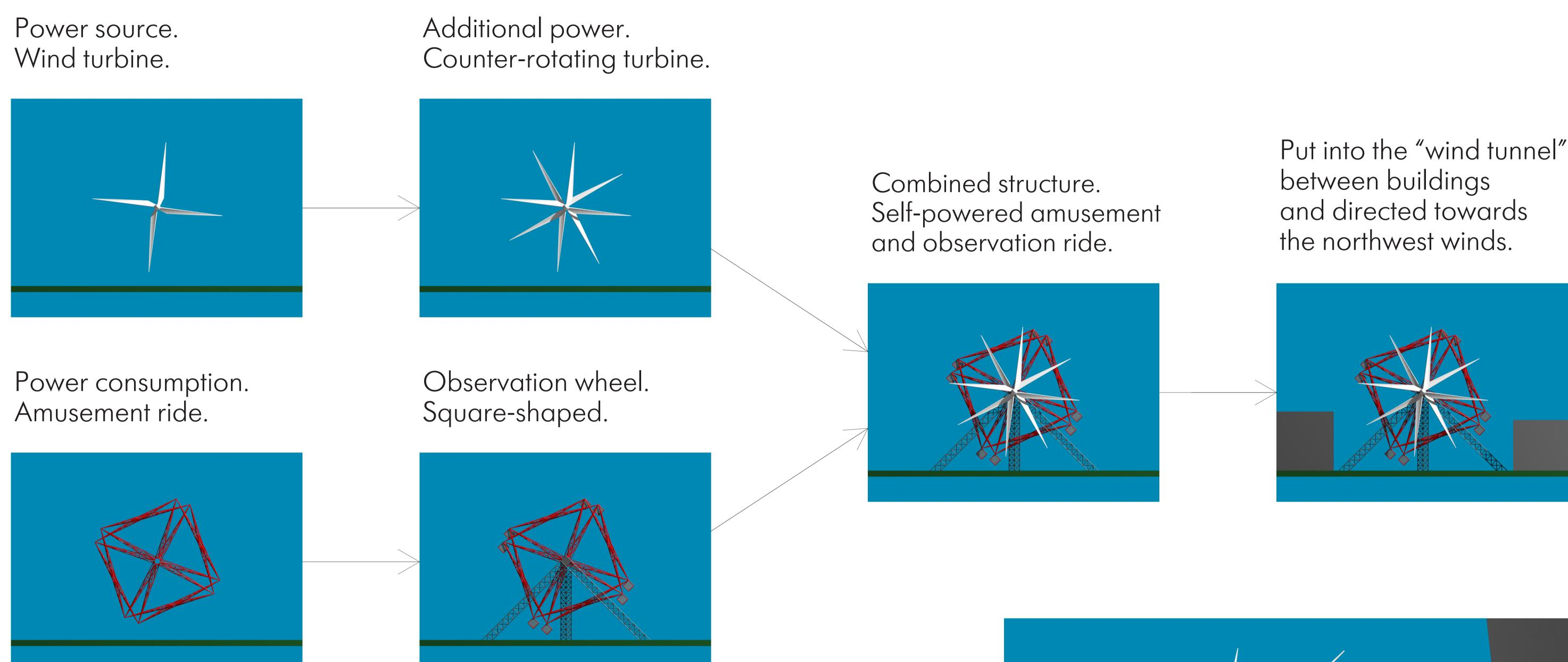
The main idea of the project is to provide direct and immediate feeling and visual effect of power, harvested from the wind by the rotational movement of rotors.
