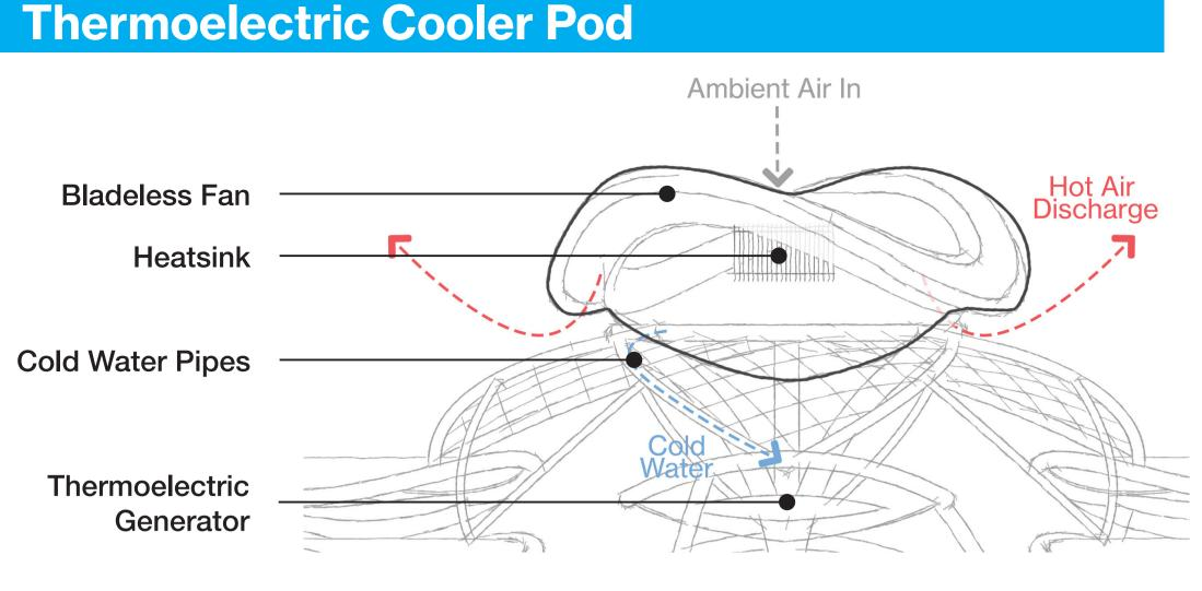
PV solar cells powers the central thermoelectric cooler pod. The high temperature and high humidity will condensed water in the cooler pods. Series of pipes are connected to the cooler pod distribute the condensed water to the bottom chamber thermoelectric generator pods.
