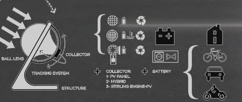
Size of one orb: 2m Energy generated by one orb: 2.2 kWh/day Total no. of orbs: 1095 Energy produced by 1 orb: 1095 x 2.2 = 2409 kWh/day Annual energy production: 2409 x 365 = 880 mWh/yr
