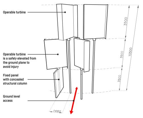
feature turbines with stainless steel rotors
