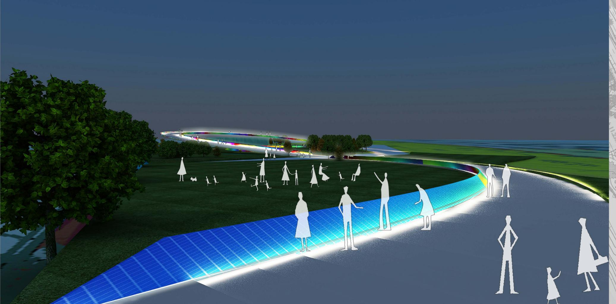
0 100 200 400 FEET First, referring to the original planning and design, redesign the footpath, and the coloured photovoltaic panel rails are added to combine the functions of the railings with the power generation functions. At night, LED lights form beautiful arcs along the trails and use the energy collected during the day to make nightscape lighting.
