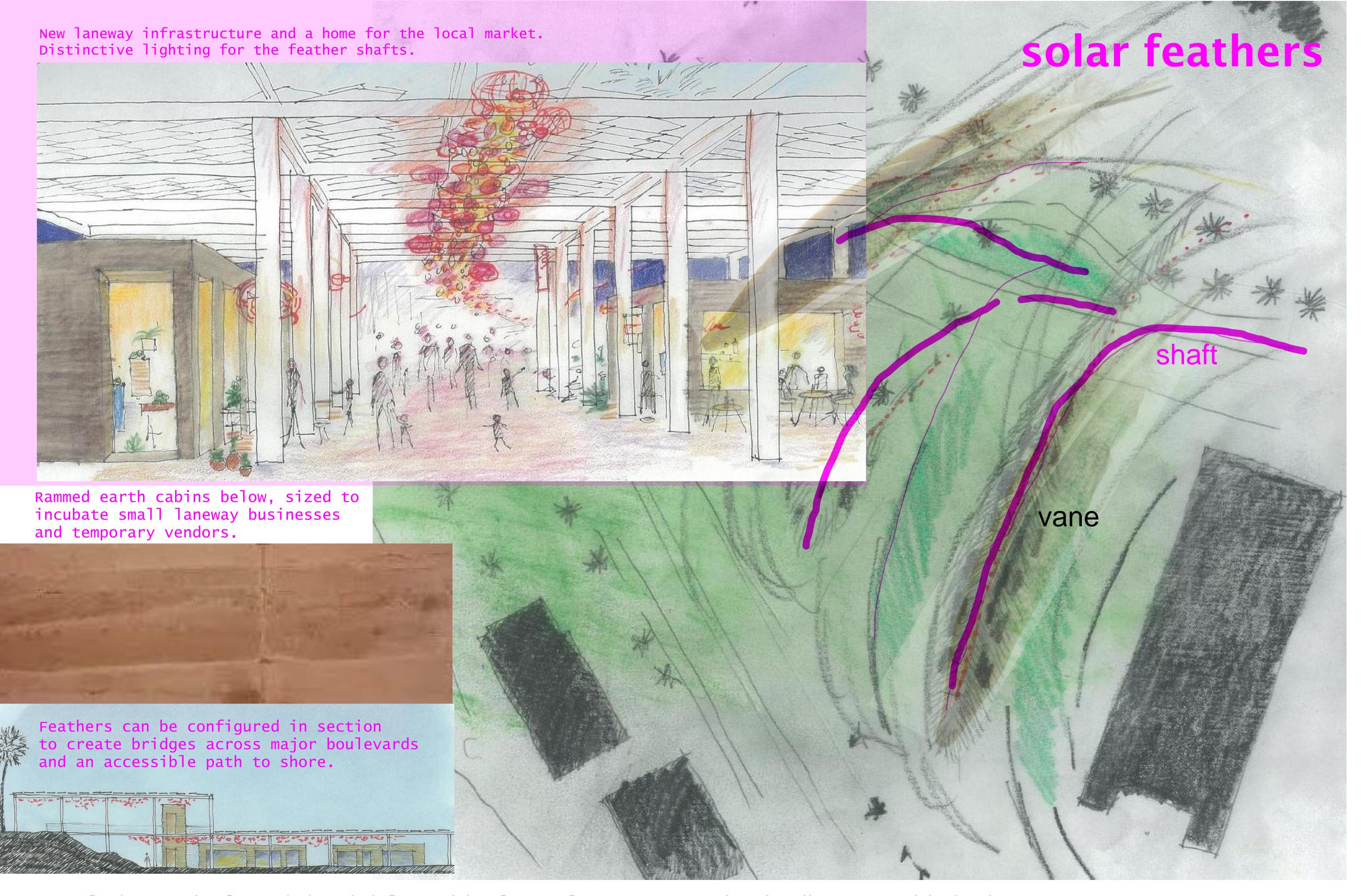
Long slender arcs in plan - shade and shelter, with solar panels on top, connecting the vibrant town with the shore. Steel structure with 196 x 99 panels in herringbone feather pattern.
