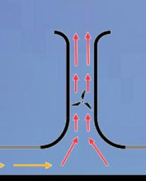
1. THE INSPIRATION OF SOL TOWER COMES FROM THE SOLAR UPDRAFT WIND TURBINE CONCEPT, WHICH LEVERAGES SOLAR THERMAL HEAT PRINCIPLES. THE AIR AT THE BASE (COLLECTOR AREA) GETTING WARMER NEEDS TO MOVE UPWARDS, WHERE THE POSITIVE TEMPERATURE DIFFERENCE (+12T) BETWEEN THE BASE AND THE TOP OF THE TOWER CREATES AIR FLOW.
