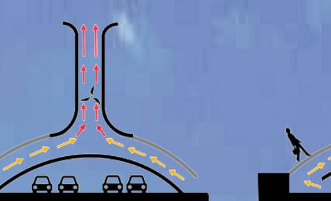
2. FROM THIS BASIC CONCEPT, OUR TEAM MODIFIED THE DESIGN WITH A HYPERBOLIC SHAPED COLLECTOR BASE. THE SHAPE OF THE BASE IS DESIGNED TO ENHANCE EFFICIENCY IN THE AIR FLOW, AND WIND VELOCITY. THE HIGH HUMIDITY OF COASTAL AIR WILL ALSO CONTRIBUTE TOWARDS A HIGHER ENERGY OUTPUT. THE BOTTOM OF HEAT COLLECTOR IS DESIGNED WITH WATER-FILLED BLACK TUBES FOR THERMAL STORAGE, WHICH WILL REJECT THE HEAT DURING NIGHT TO MAINTAIN ROUND THE CLOCK TURBINE OPERATION AND POWER GENERATION.
