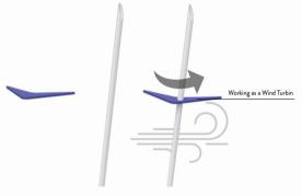
When the wind blows, the boomerangs spin about the metal axis, like a wind turbine, and the sculpture receives the wind energy. The wind energy generated by the boomerangs, which are placed in different heights and positions is about 160MWh energy in a year. The metal path is also made of renewable steel.
