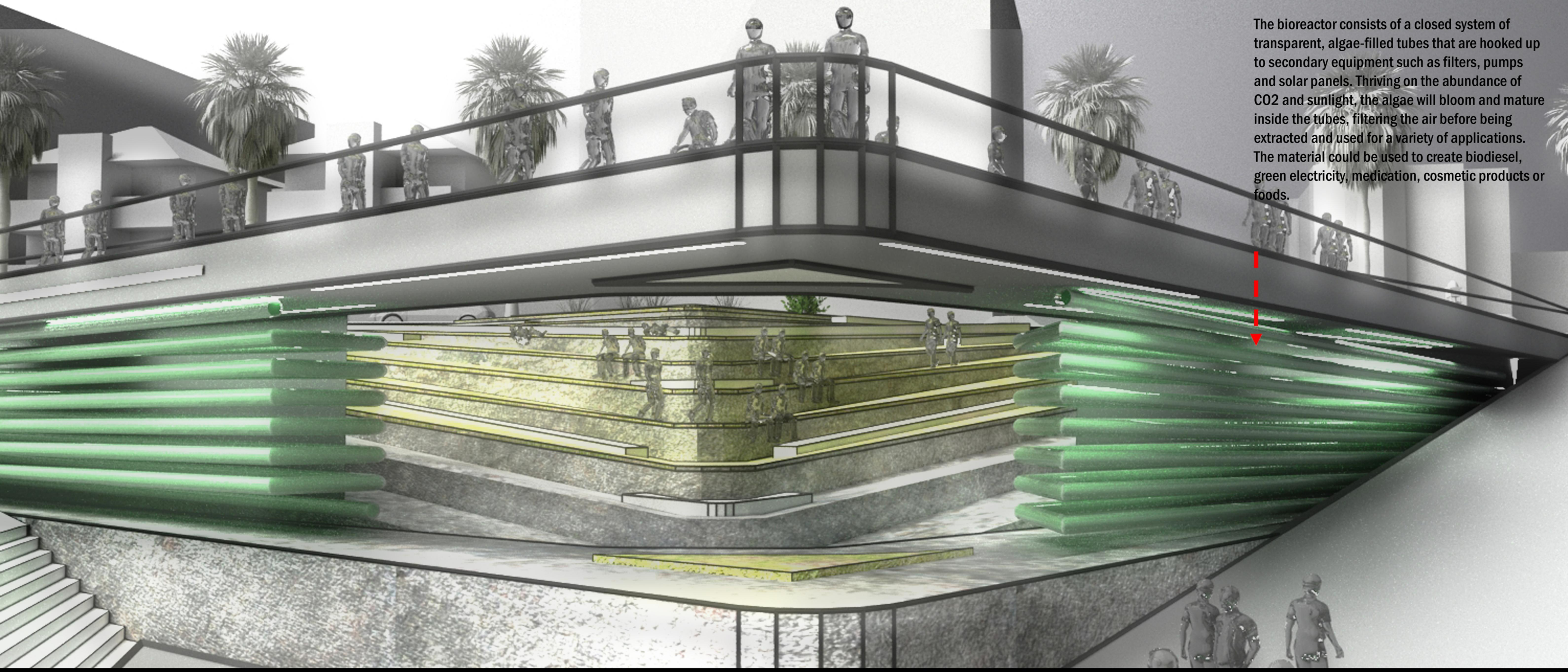
The bioreactor consists of a closed system of transparent, algae-filled tubes that are hooked up to secondary equipment such as filters, pumps and solar panels. Thriving on the abundance of CO<sub>2</sub> and sunlight, the algae will bloom and mature inside the tubes, filtering the air before being extracted and used for a variety of applications. The material could be used to create biodiesel, green electricity, medication, cosmetic products or foods.
