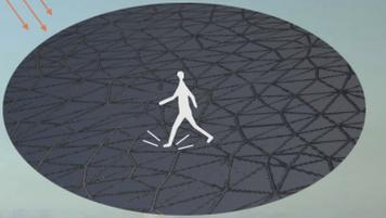
The promenade pavement combines two technologies to generate energy: an overlay of triangular solar tiles over electro-magnetic generators.
