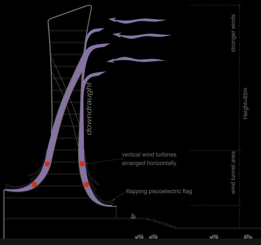
Principle sketch: -Bottom of the tower with energy harvesting machines -Elevation with structure similar to whale's skin for more condensed air flow Principle section:
